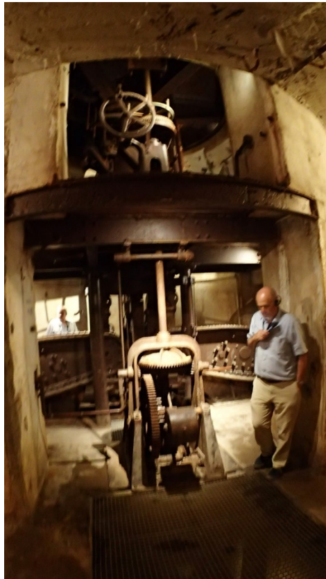
Mechanism for lowering and raising a big gun after each firing. This was the first mechanized, industrial war.
